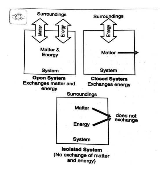
All the physical and chemical processes taking place in open in our daily life are open systems because these are continuously exchanging matter and energy with the surroundings.
