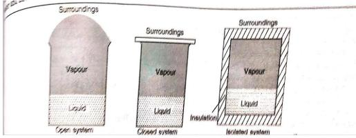
• (I) Open system: A system which can exchange matter as well as energy with the surroundings is called an Open system. For example, hot coffee in an open flask is an example of open system because it can gain or loss matter as well as energy.
